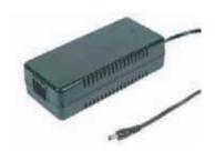
Input: 95~264VAC Output: 80W, 48 VDC, 1.66A AC inrush current: 40A at 230VAC Overload Protection: Hiccup mode, auto-recovery Over Voltage Protection:
